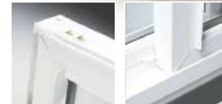
Each sliding window operating sash features two sets of solid-brass tandem rollers to ensure smooth, effortless window operation (left). Sash limit-locks allow fresh air ventilation (right).
